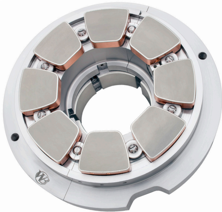
Combination tilt pad bearing with copper-backed babbitt thrust pads and steel-backed babbitt journal pads.
