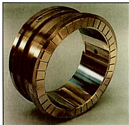
Machining stage of thick wall 4 lobe bearing for a 40MW gas turbine reduction gearbox.
