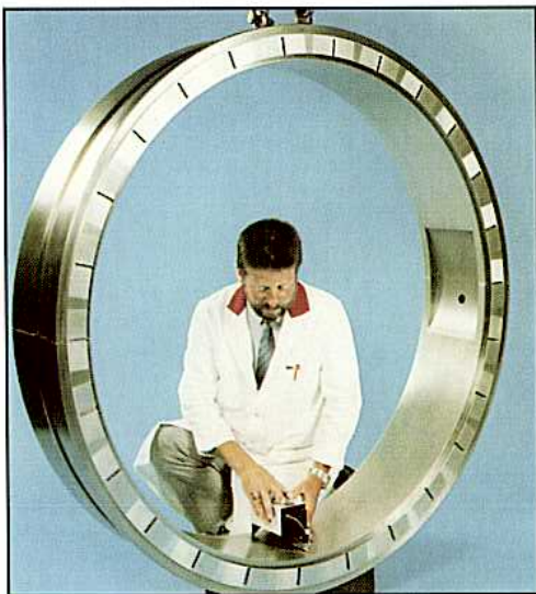
1500mm journal bearing with taper land thrust face for 2.5MW marine alternator drive.
